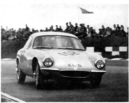
OTUS realise the advantages in using this integral fibreglass chassis/body structure. Beautifully finished, exceedingly light and offering superior heat and noise insulation.
