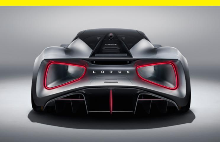
The most striking element of the Lotus Evija is its exterior. From every angle the full carbon fibre bodywork is stretched taut, appearing shrink-wrapped over the mechanical components. Crouching low to the ground, with a ride height of just 105 mm, the pronounced muscular haunches envelop the teardrop cabin that sinks between them.
