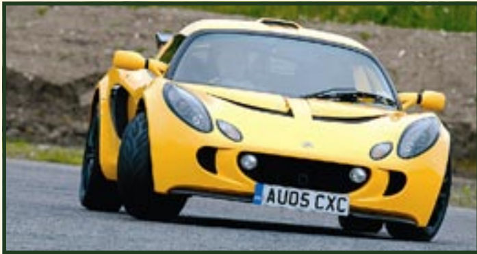
Understeer, where the front tyres are working at a greater slip angle than those of the rear.
