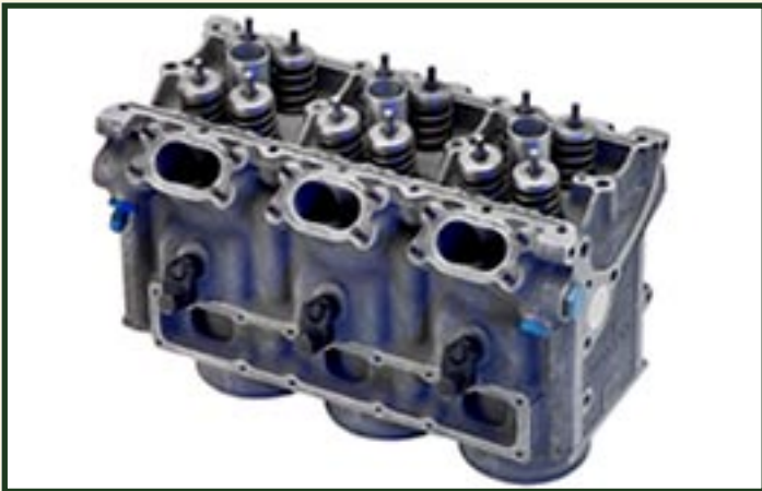
Research racing engine monoblock. Note direct injector position under the intake ports; these are in a position which would usually be occupied by a cylinder head gasket
