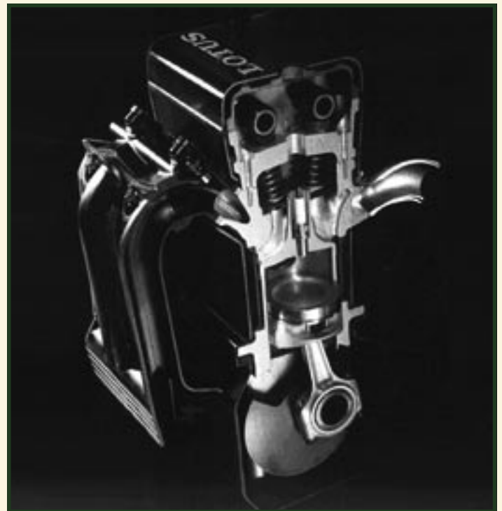
Lotus 'Jewel' concept engine: monoblock construction, magnesium ladder frame and composite water jacket, oil drains and cam cover
