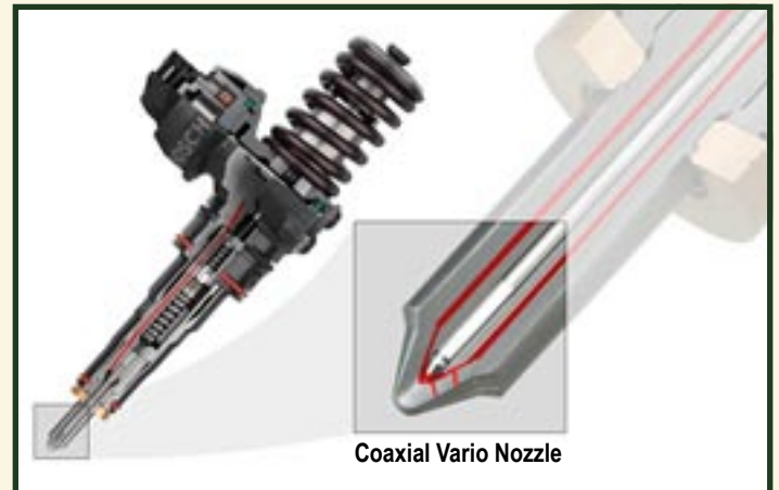
Bosch's 4th generation Unit Injector System Source: Bosch
