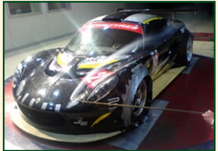
Wind tunnel testing the 2006 car
