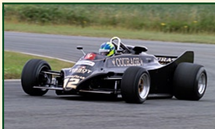
Lotus Type 88 – innovative twin-chassis outlawed by regulation changes
