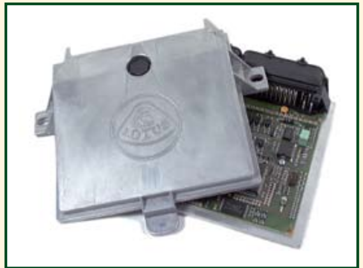
The T4 controller - Lotus' first use of software safety analysis in the 1990s
